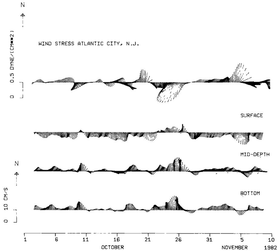
Fig. 1. Time series vector plots of low-pass filtered wind stress at Atlantic City, New Jersey, and current in the Delaware Estuary at three depths from a current meter mooring in 9 m of water. Vectors are drawn toward the direction of motion. North (upward on the figure) is nearly landward along the estuary locally. Wind stress and current magnitude scales are shown on the left. From Wong and Garvine [1984].
