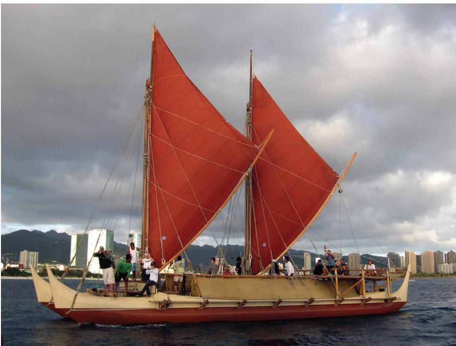
FIGURE 2-3 The Hokule'a . This vessel is a reproduction of the double-hulled voyaging canoes that the Polynesians used to explore and colonize the Pacific.
