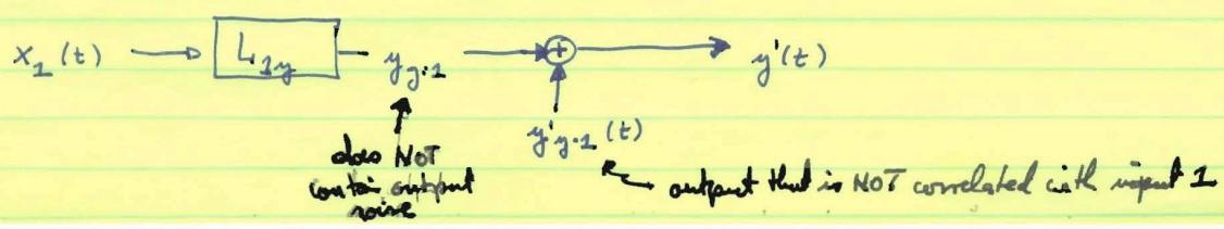
The "conditioned" system has exactly the same form as the "ordinary" system as both the input and output in the "ordinary" system are replaced by their "conditioned" equivalents. The "conditioned" input does not go to the raw output but to the "conditioned" output. Nevertheless, the cross-spectra
