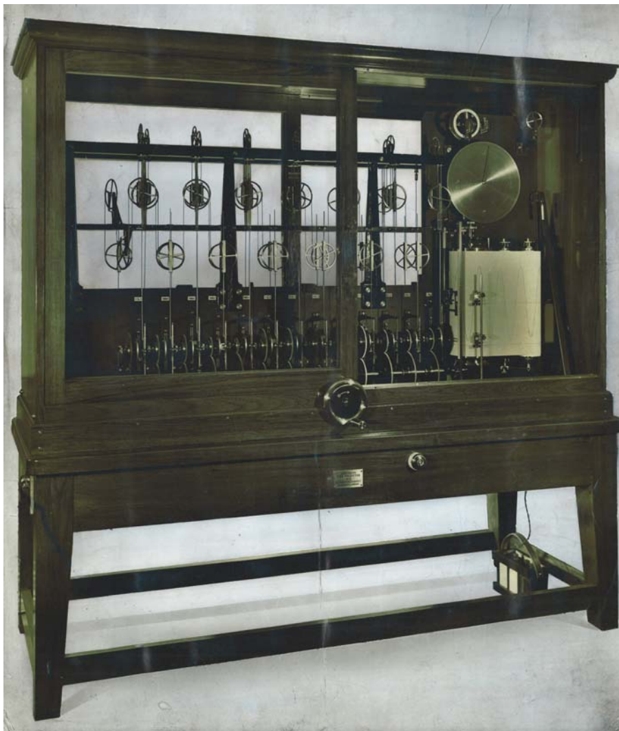
Figure 2. Kelvin's tide machine, the mechanical calculator built for William Thomson (later Lord Kelvin) in 1872 but shown here as overhauled in 1942 to handle 26 tidal constituents. It was one of the two machines used by Arthur Doodson (above) at the Liverpool Tidal Institute to predict tides for the Normandy invasion. (Photos courtesy of Proudman Oceanographic Laboratory.)
